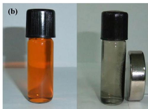
Fig. 5. (a) Magnetization curves of porous FeCo/carbon nanocomposites FeCo/C-1, FeCo/C-1.5, and FeCo/C-2 at room temperature, respectively; (b) magnetic separation from MO solution for Fe 2 CO 3 /carbon nanocomposites under an external magnet.
